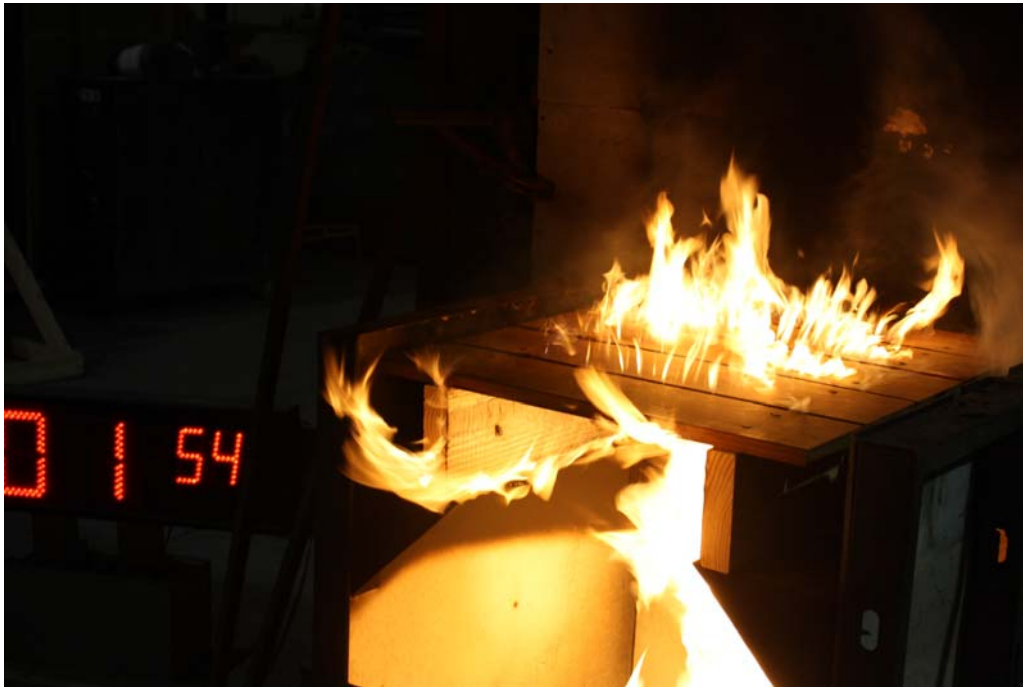
Part A – Underflame Test: Example of Specimen During Test
