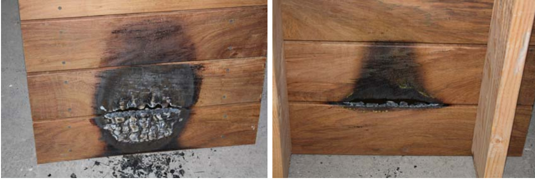
Burning Brand – Example of Deck Post Test
