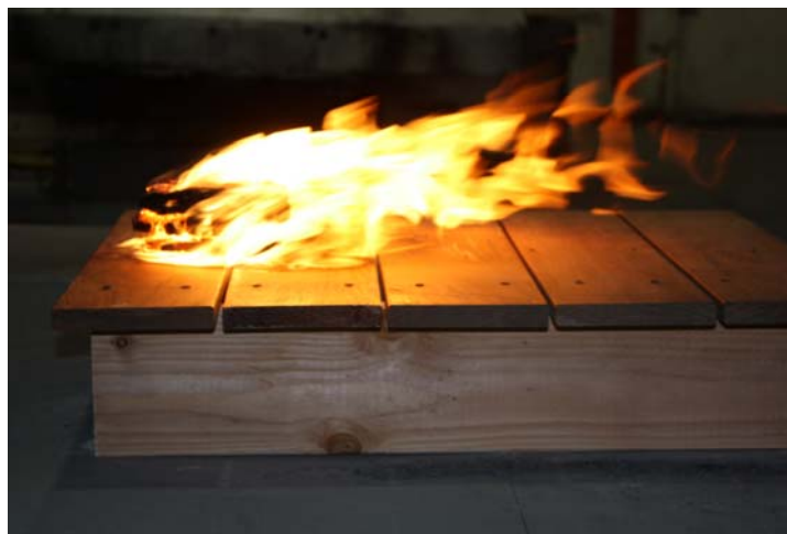
Burning Brand Test – Example of Deck Surface During Test
