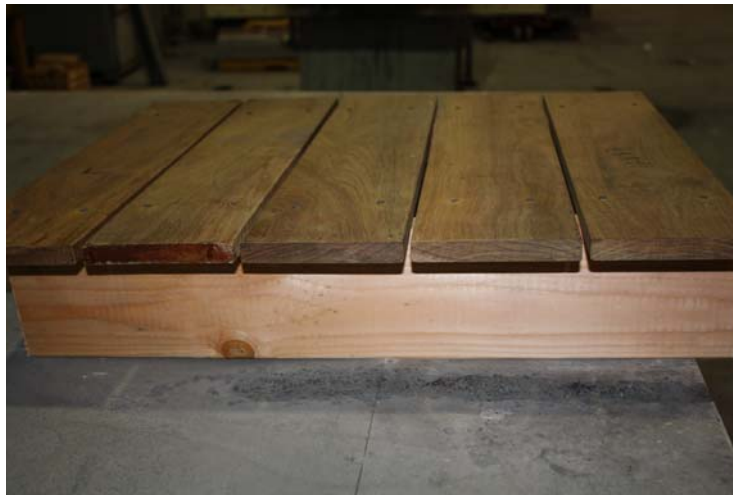
Burning Brand – Example of Specimen Prior to Test
